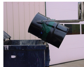
Pivoting drum for ease of dumping.
