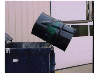
Pivoting drum for ease of dumping.
